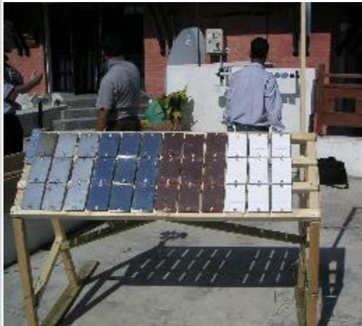
Corrosion monitoring track installed in Kathmandu, Nepal
